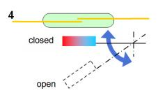
A magnet in **swiveling motion** to the reed switch. The magnet must be moved at a large angle so that the switch closes once.
